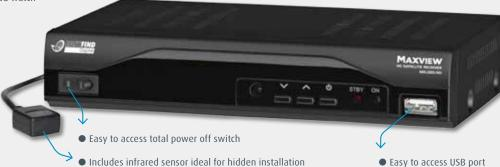
Includes infrared sensor ideal for indden installati
