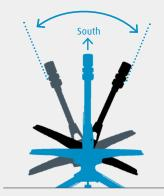
Limited satellite zone. Reduces margin for error, so locking on to the correct signal is quicker and easier.
